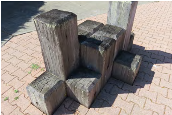
Weathered wood sculptures exhibiting checking, general soiling, and biological growth
